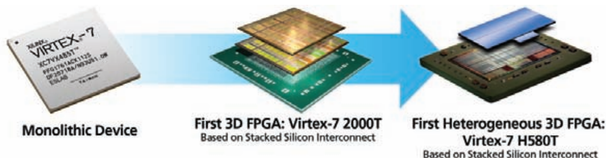
Figure 1 – Xilinx 3D SSI technology forms the foundation for the Virtex-7 H580T, the world's first heterogeneous FPGA. It marries 28-nm FPGA logic slices and a dedicated 28-Gbps transceiver die on a silicon interposer.
