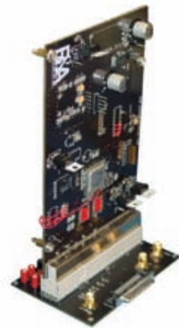
Figure 1 – The Xilinx Virtex-5, XC5VLX30 test board
