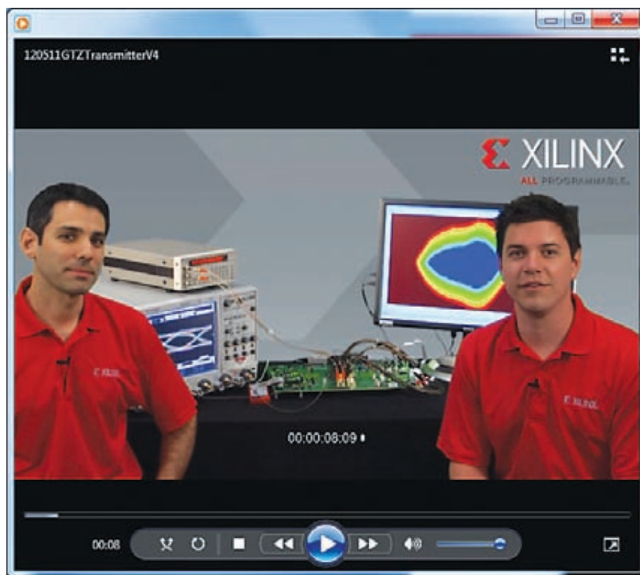
Video: A Virtex-7 H580T device demonstrates its ability to deliver the eye and jitter characteristics necessary to reach the performance required to interface to CFP2 optic modules.
